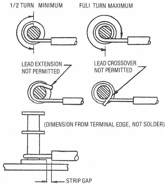
Figure 5.11. Soldering to Turret Terminals
