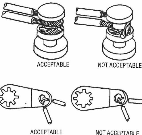
Figure 5.2. Terminal and Lug Wiring
