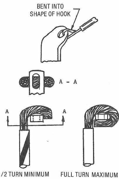
Figure 5.18. Terminating Large Diameter Wire
