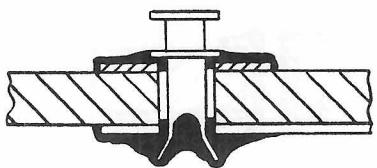
Figure 5.22. Soldering Flanged Terminals
