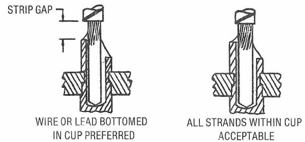
Figure 5.14. Soldering to Cup Terminals
