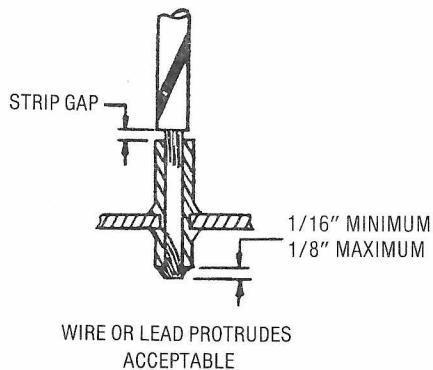
Figure 5.15. Soldering to Feed-thru Terminals
