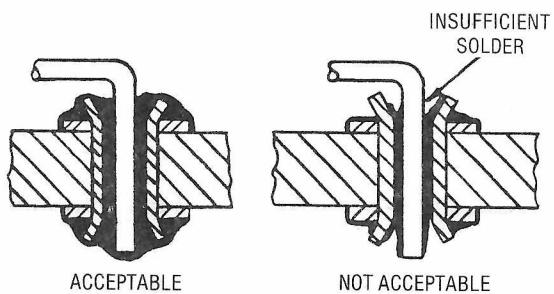
Figure 5.21. Soldering to Eyelet Holes
