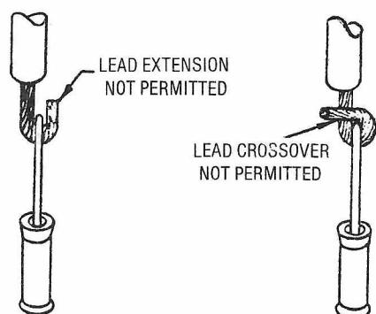
Figure 5.13. Soldering to Hook and Pierced Terminals
