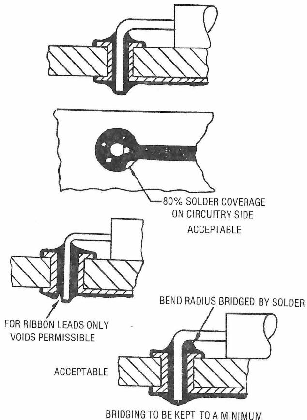
Figure 5.20. Soldering Plated-Thru Holes
