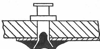
Figure 5.24. Soldering Standoff Terminals
