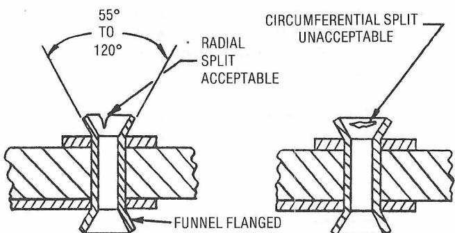
Figure 5.25. Mechanical Assembly of Eyelets and Terminals
