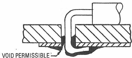
Figure 5.23. Soldering Unplated Holes
