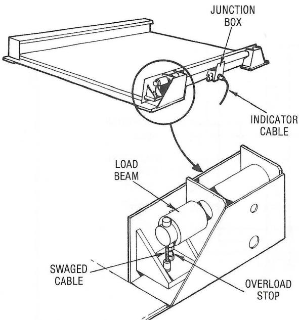
Figure 3.20. Typical Low Profile Scale
