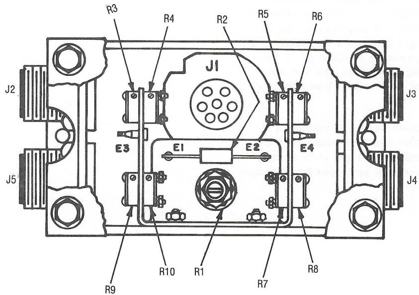
Figure 3.21. Junction Box/Schematic/Low Profile/Deck Scale
