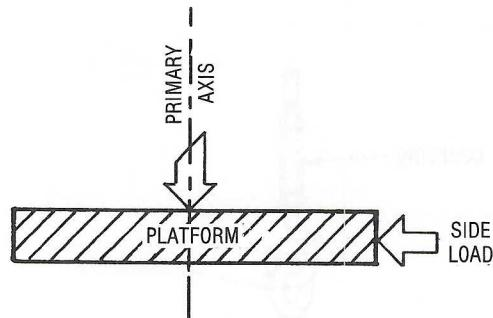
Figure 3.18. Graphic Illustration/Side Load
