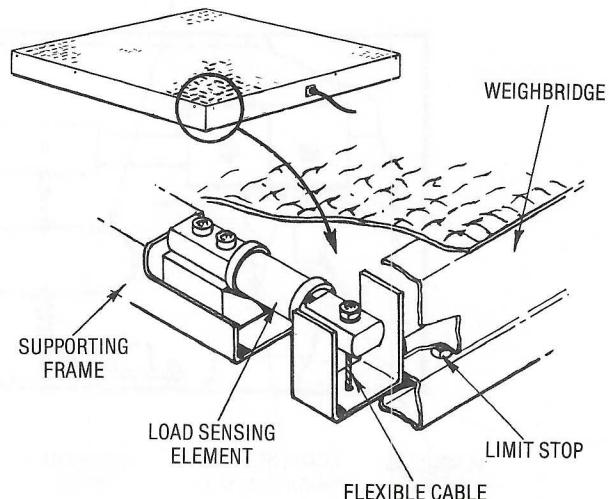
Figure 3.19. Typical Deck Scale
