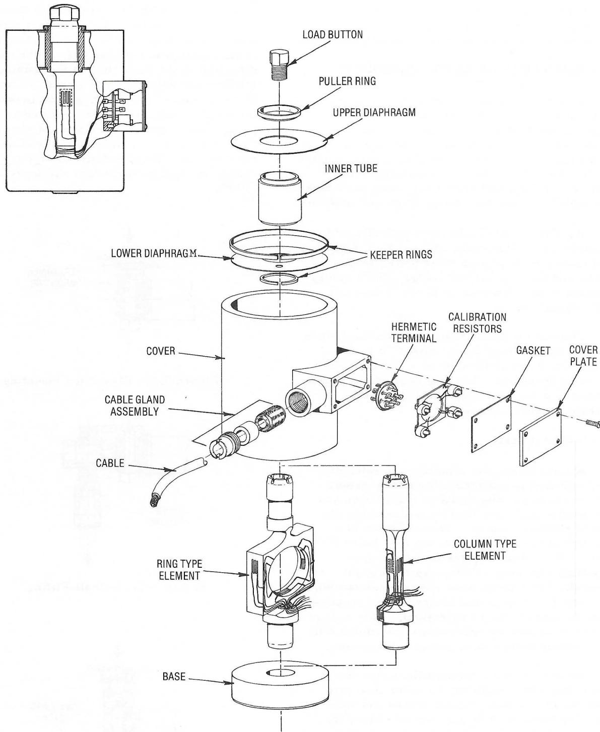
Figure 3.7. Typical Load Cell Construction
