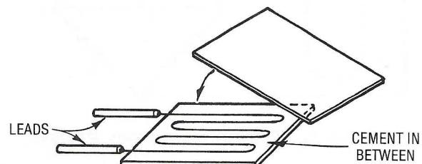
Figure 3.1. Strain Gage
