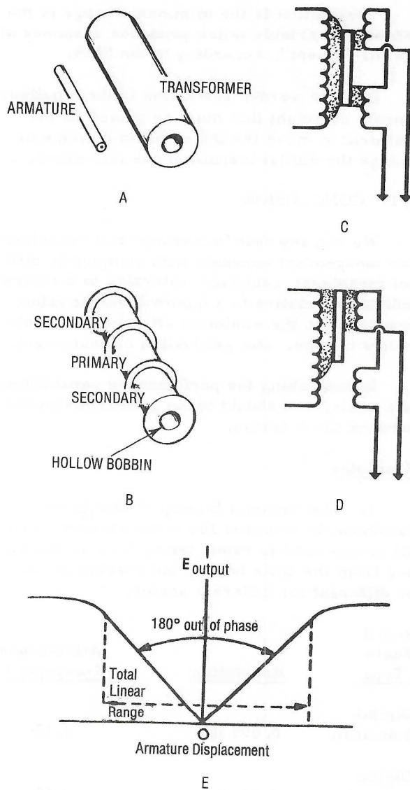
Figure 3.12. Linear Variable Differential Transformer (LVDT)
