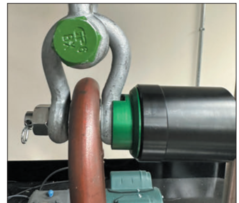
Figure 2 Morehouse Prototype Shackle Load Pin Test.
